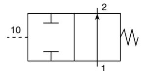
Valve actuated by pneumatic signal applied to port 10.
