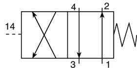
Valve actuated by pneumatic signal applied to control 14.
