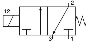
Valve actuated by electrical signal applied to control 12.
